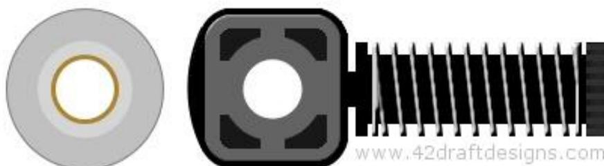
The side/side endlink is square and accepts the round bushings marked B6SS51. The pin diameter is roughly 8mm. The side/side endlink connects directly to the metal side/side linkage.
